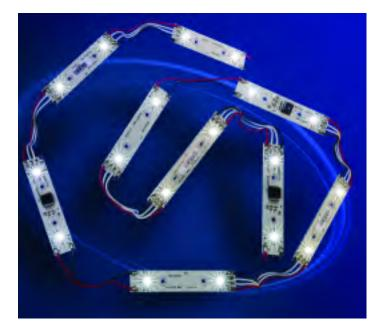
The OSRAM SYLVANIA HF<sup>2</sup>Chain LED module offers alternatives to traditional neon sources. The main advantage of the LED module over neon sources is reduced manufacturing and maintenance cost, durability, and small size.
